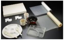
PHBH is produced by a microorganism fermentation process, in which plant oils and its fatty acids are used as a primary raw material.
